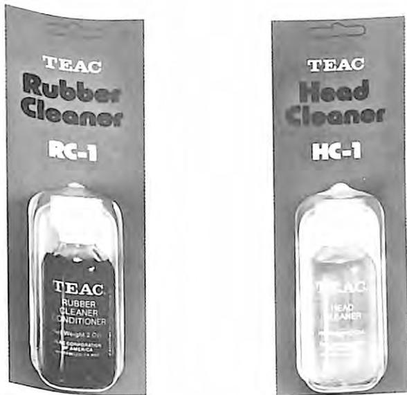
Using the right chemicals is important because strong solvents can dissolve the binder that holds the head laminations together. Isopropyl alcohol can leave a residue and is not always adequate for cleaning desposits from modern tape formulations. Beware of rubbing alcohol; while it is isopropyl, it also contains oil and water that leave a heavy film on the heads. TEAC HC head cleaner is formulated to clean tape heads, tape guides, and capstans without leaving a film or damaging head integrity.
